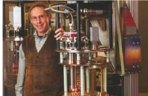
High Precision Devices' president Bill Hollander stands next to a cryostat, a cylindrical cold chamber capable of cooling to a temperature of about three-hundredths of a degree Kelvin. The company makes equipment using core technologies of precision mechanics, optics, vacuum and ultra-high vacuum, electronic sensing and control, and cryogenics.
