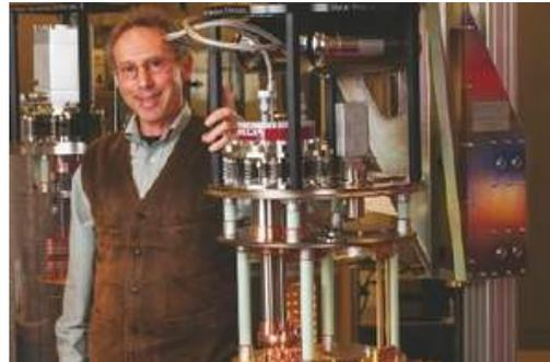
High Precision Devices' president Bill Hollander stands next to a cryostat, a cylindrical cold chamber capable of cooling to a temperature of about three-hundredths of a degree Kelvin. The company makes equipment using core technologies of precision mechanics, optics, vacuum and ultra-high vacuum, electronic sensing and control, and cryogenics.
