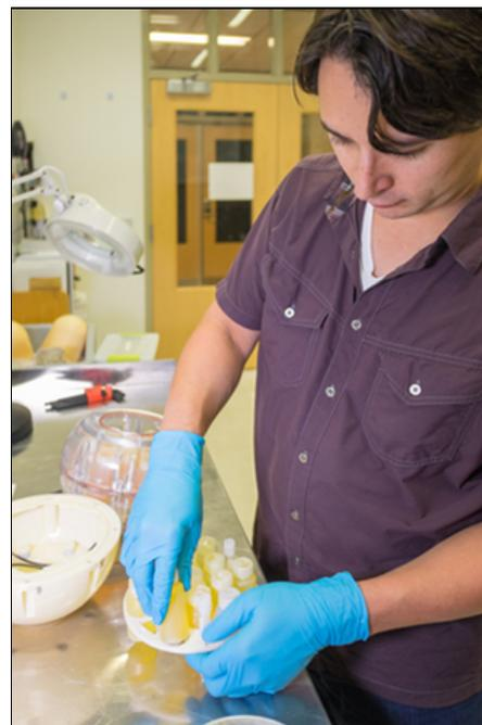
NIST physicist Michael Boss with his prototype diffusion phantom for calibrating magnetic resonance imaging (MRI) scanners. The phantom contains 13 vials of polymer solutions that represent various rates of diffusion of water molecules. Diffusion rates are used in diagnosing traumatic brain injury and neurodegenerative diseases. The phantom has been commercialized and is being used in clinical trials.
