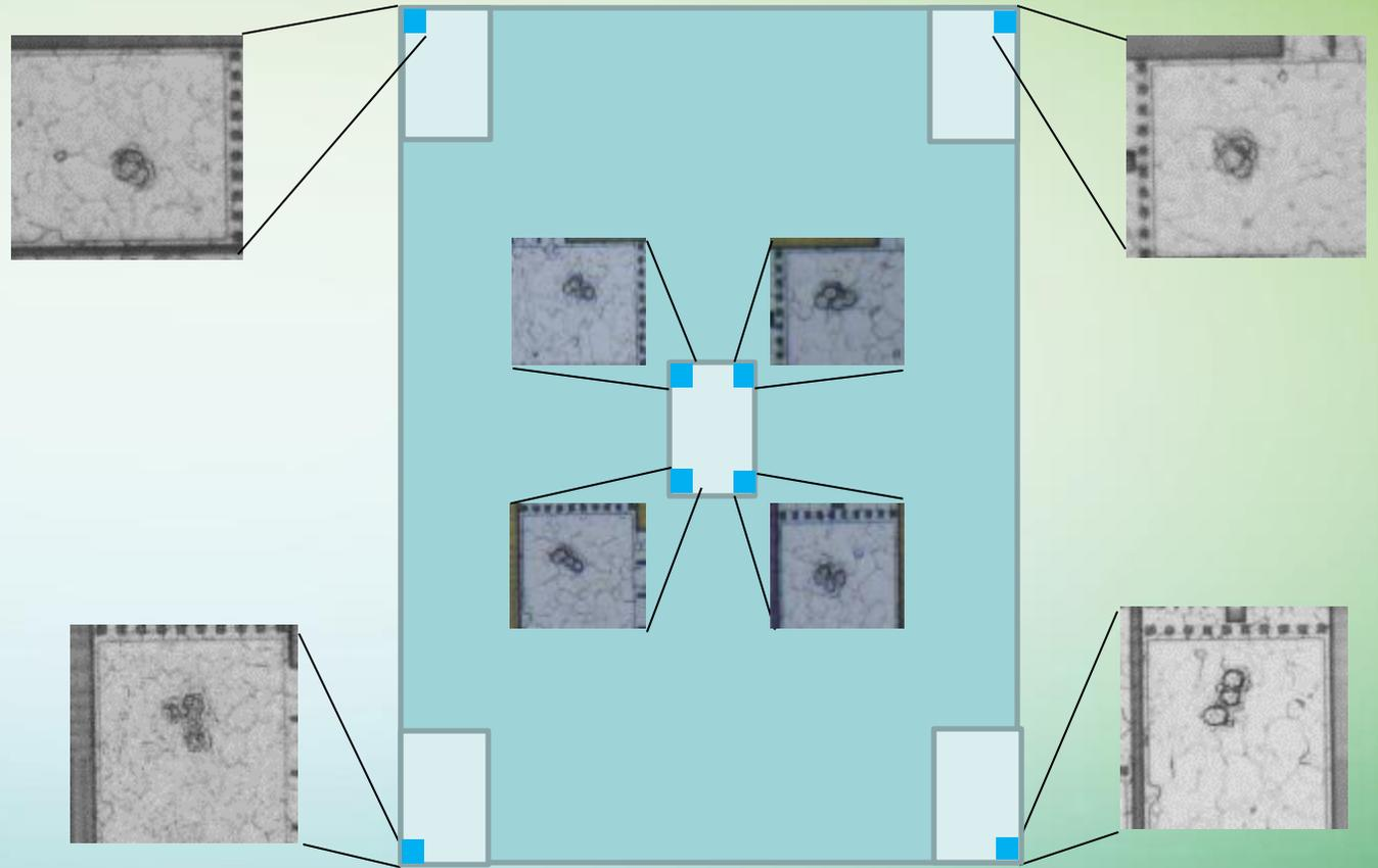
Architecture demonstrating very stable scrub mark placement from -40°C to 150°C
