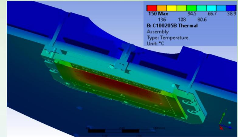
Thermal model of a probe card with prober chuck temperature set at 150°C
